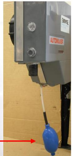
(c) To send data. Point the data transmitter at the black infrared receiver in the bottom window. If this is done in direct sun light, you will need to be closer to the receiver and shade the receiver from direct sun light.
