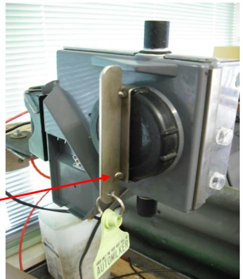
4. Use Automilker spanner to undo sensor cap.
